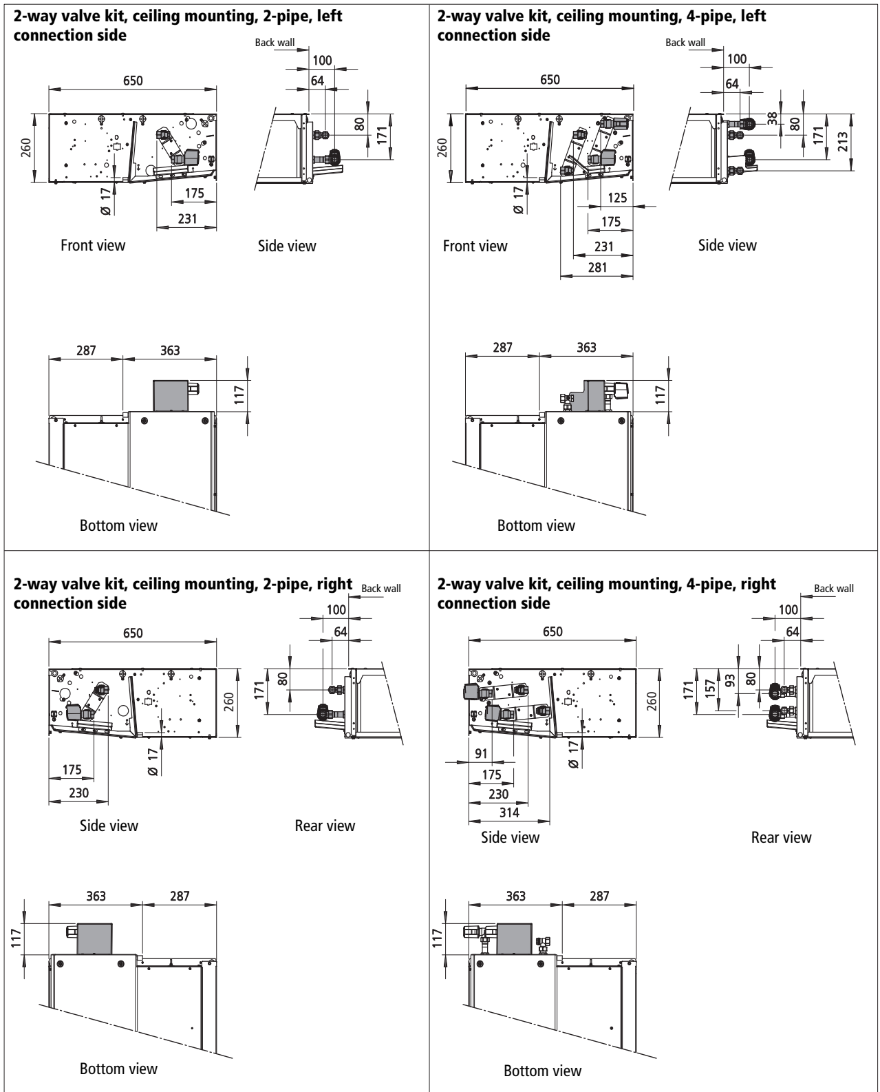
Fig. 12: Dimensions 2-way valve kit (ceiling-mounted version)
