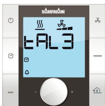
View "Real-time clock faulty in the KaController" (Alarm tAL3 shown)
